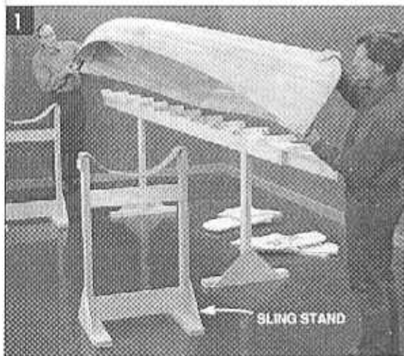
REMOVE THE CANOE from the strongback and place it on sling stands, which support it while you work on the inside of the hull and the trim.
